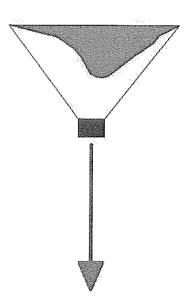
Parachute not yet been released Maximum downwards pull Zero air resistance
