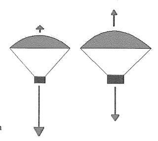
After it has been released the parachute gradually decelerates since there is air resistance acting upwards on it...
