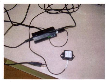
The hardware used to measure the accelerations when braking on the bicycle. The small sensor would be mounted on the handlebar, whilst the rest would be in the backpack.
