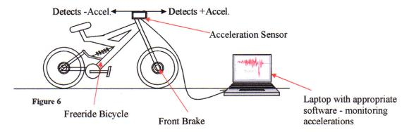
A test run is carried out in order to explain and clarify the various sections of the graphs generated:
