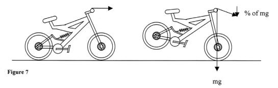
This implies that for all the readings where the bike starts to tip-over the average acceleration will be including part of the acceleration due to gravity. This is a systematic error and thus will shift all the values to be more negative than the supposed prediction.
