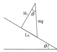
$L_{\rm N}$  represents the force accelerating the bike down the slope due to the acceleration from gravity. In order to calculate this I simply use trigonometry and know that
