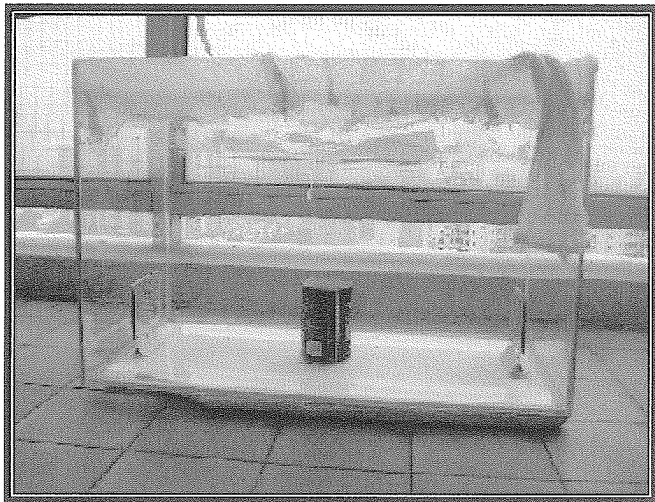
Figure 19: The control, set up between two sticky card lures only on either side of the tank with the food tin containing mosquito larvae in the centre.
